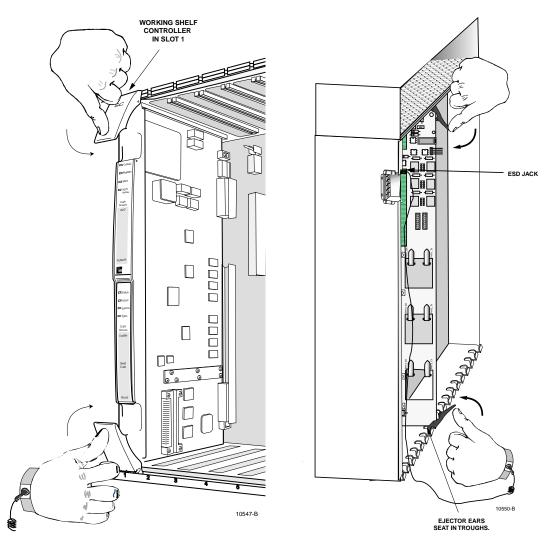
Figure 777-2. Example of Seating a Front Access Card or EIM in a Shelf
